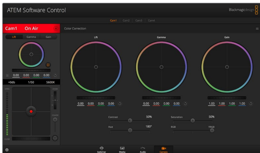
Click on the DaVinci Resolve primary color corrector button to expand the color correction window and adjust settings
