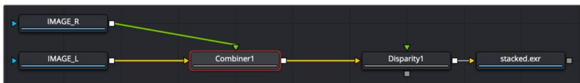
Left and right eye images are connected into a Combiner node to generate a stacked stereo image.
