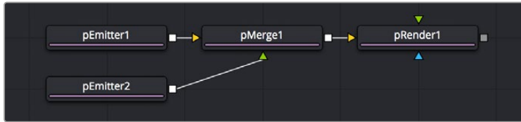
Compositing two pEmitter nodes to create a compound particle system, combining two kinds of particles together
