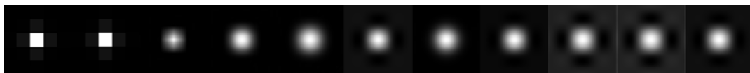
Resize Filters from left to right: Nearest Neighbor, Box, Linear, Quadratic, Cubic, Catmull-Rom, Gaussian, Mitchell, Lanczos, Sinc, and Bessel
